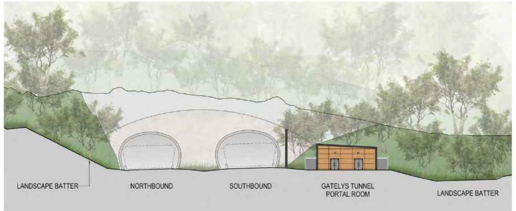
GATELYS ROAD - TUNNEL EQUIPMENT ROOMS - SITE ELEVATION
