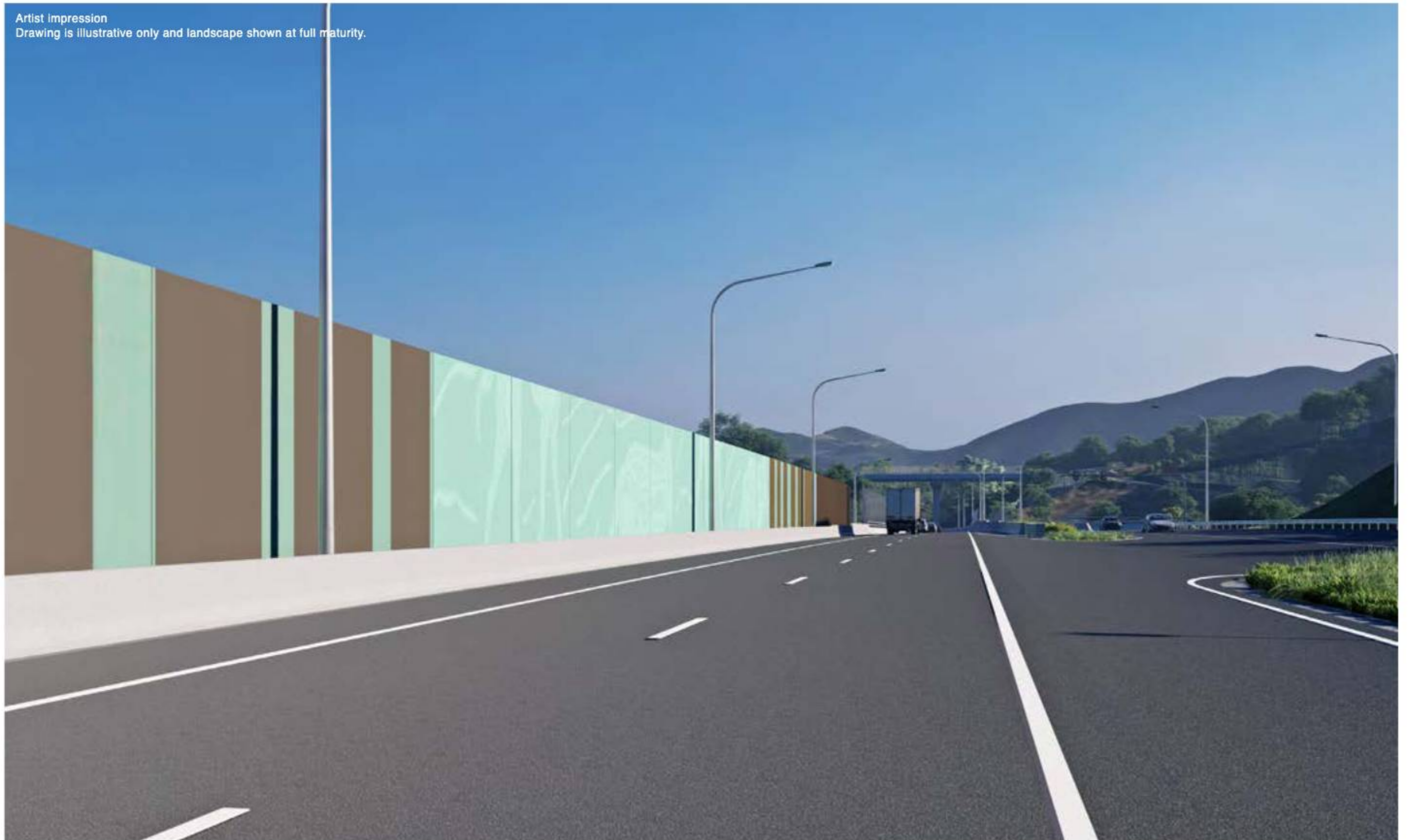
Figure 187: View of noise wall - southbound exit of Shephards Lane Tunnel southern portal
